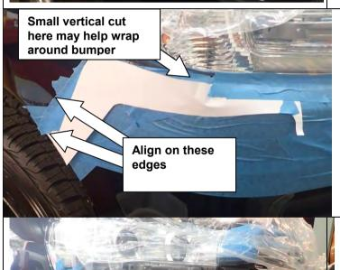
11. Ensure template is correctly positioned along the edge of the bumper both at the front quarter panel as well as along the wheel arch. Mark along cut edge with a marker.
