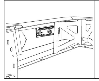
57. Fit the small plastic grommets to the bar and attach the combination LED lamps to the bar using the screws provided with the lamp kit.
