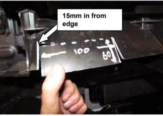
31. Now on the upper face of the power steering shroud mark and cut as shown
