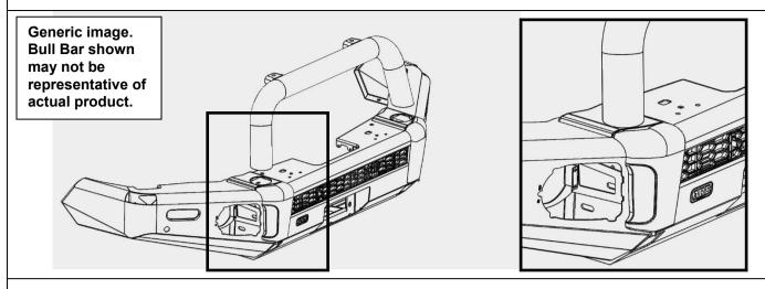
56. Fasten top tube to the bar using 4 x M10 SEMS Bolts. Adjust position of top tube left/right until it sits central on the bar and the rear buffers are positioned correctly. Tighten M10 SEMS Bolts to specification. Tighten Rear buffer screws.
