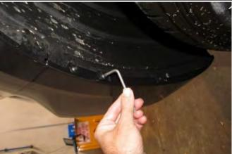
2. Remove inner guard bumper retaining screws three per side using T30 Torx key.
