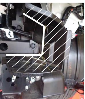
Mark out a second line to meet up with the line in the previous step. Cut the air deflector on the LHS of the vehicle using a multi tool or similar. Shaded area shown must be removed.
