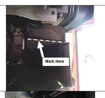
28. Mark the lower section of the air scoop for the power steering radiator as shown. This is for trimming to clear the mount brackets.
