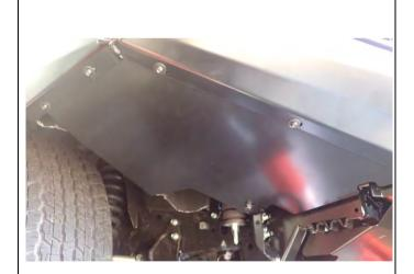
95. Trim the fender liner end flush with the splash panel face as shown. Then tuck the remaining wheel liner inside the wing panel return.
