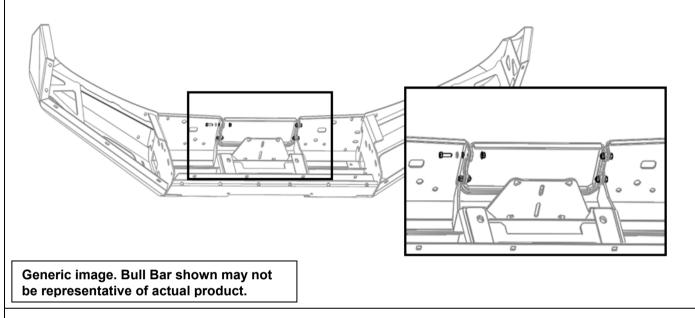
42. Fit the number plate bracket to the top face of the lower-centre pan on the bar using 3 x M6 x 20 hex bolts, spring washers, flat washers and flange nuts.
