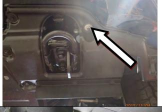
4. When removing lower trim panels, a plastic nut located on each side will need to be prized open with a small flat blade screwdriver to assist removal.
