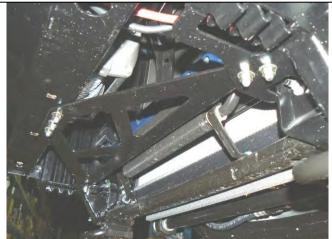
76. Loosely fit the cross brace to underside of lower pan and on top of gussets of mount brackets. Use M10 x 30mm SEMS bolt and flange nuts.
