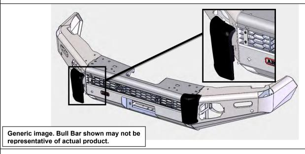
52. Ensure each buffer sits flat against the face of bar. Secure wing side using retaining clips. Secure inner side using the angled cup washers, flat washers and screws.
