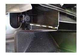
29. Now mark along the lower bend as shown, now cut the shroud along the marked edges as shown
