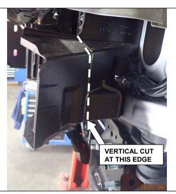
32. Mark out a vertical cut line on the LHS air deflector.
