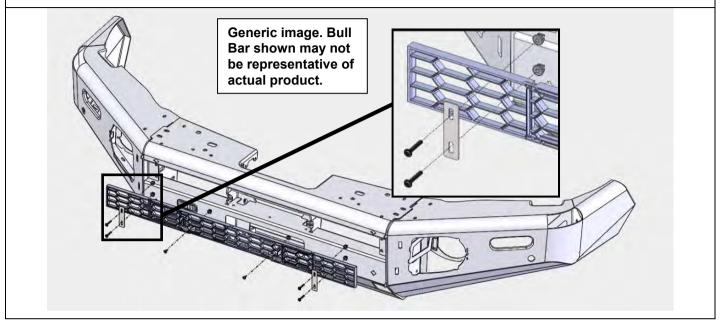
51. Place each of the front buffer sections onto the bar as shown. Ensure that the 2 lugs and 2 screw bosses pass through the holes in the bar.
