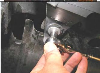
5. Remove lower bumper retaining screws.
