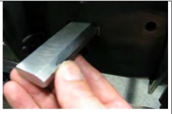
58. Insert clevis nut into rectangular hole in the inboard face of chassis, ensuring the threaded end is inserted first.
