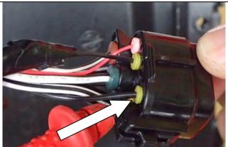
72. If installing driving lights, the high beam signal can be tapped into on the passenger side of the vehicle using the black wire on the black plug shown.
