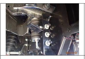
92. Fit both wing panel brackets to the higher holes in the outside of the mounting brackets using M8 bolt, washer, spring washer and flange nut.
