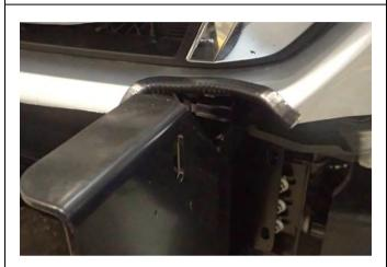
66. Fit pinch weld to the cut edge of the bumper as shown.
