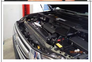
6. Remove plastic engine bay cover above grille area and set aside. Press down on centre of plastic plugs with small screwdriver or similar to release.
