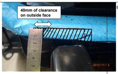
65. The Mounting brackets will contact the bumper, mark a rectangular cut on the bumper to ensure that there is a minimum of 25mm of clearance between the mounting bracket and the bumper. 40mm clearance is required on the outside face of the mount. Remove shaded area of bumper.
