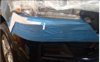
Apply wide masking tape along bumper as shown, then having cut out template, apply to outer corner of RHS bumper as shown. Align with edge of quarter panel, wheel arch and underside of headlight.
