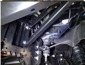
77. Loosely fit both left and right wing braces to inside of wings and mount brackets. Use M10 x 30mm SEMS bolt and flange nuts.
