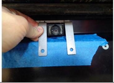
50. Position camera and bracket on the Beaver panel. Check function of the camera, when the camera is positioned correctly make and drill 2 x Ø7.0 mm holes. Secure camera and bracket to the beaver panel with 2 x M6 cap head screws, washers and nuts.
