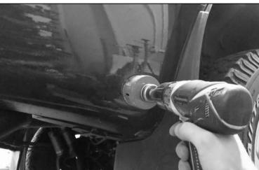
86. Using a Ø70mm hole saw, drill through the rear side panel using the mark from the previous step as the centre point of the hole.
