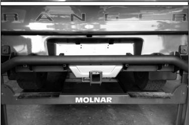
50. Position the bar so there is even spacing to the vehicle and tighten all fasteners to the specified torque.
