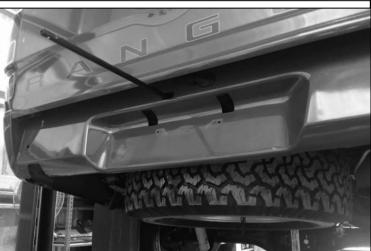
11. Remove the spare wheel from beneath the tub using the wheel nut wrench and jack handle pieces supplied with the vehicle. Insert as shown through the access slot above the number plate position and rotate counter-clockwise to release the wheel.
