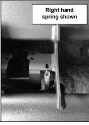
41. Using pliers, stretch the free end of each spring up to the bracket on the RSTB as shown.
