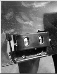
91. Place a wing double nut plate inside the middle bracket of each Ranger wing as shown.
