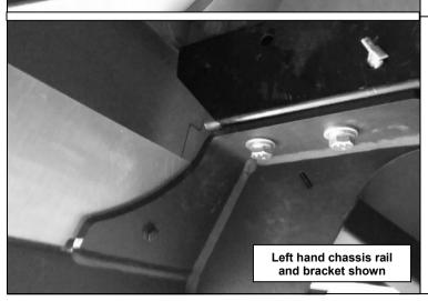
47. Place 2 M12x1.25x40 (fine pitch) hex head bolts, 2 M12 spring washers and 2 M12 flat washers per chassis rail through the RSTB plate as shown. Attach using the chassis double nut plates placed inside the chassis rails in the previous step. Leave finger tight at this stage.
