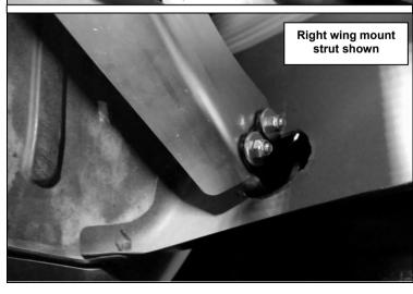
100. Pass the front bracket of each Ranger wing through the Ø70mm hole in the tub and fasten to the wing mount strut using 2 M8x1.25x25 hex head bolts, 4 M8 flat washers and 2 M8 nyloc nuts. Leave bolts finger tight at this stage.
