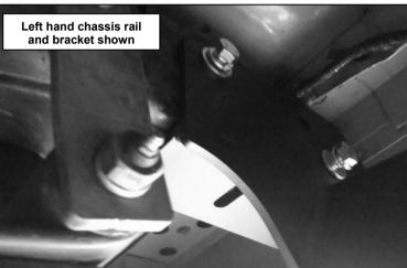
45. Fix the vertical plates of the RSTB over the threaded holes in each chassis rail using 2 M12x1.75x40 (coarse pitch) hex head bolts, 2 M12 spring washers and 2 M12 flat washers per chassis rail. Leave finger tight at this stage.
