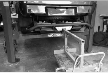
44. With the assistance of other people or a lifting device, lift the RSTB up beneath the chassis rails aligning the threaded holes in the side of the chassis with those in the vertical surfaces of the RSTB.
