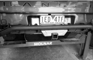
63. Tidy and fasten all wiring using cable ties and the slots in the RSTB brackets, as well as existing fastening locations.
