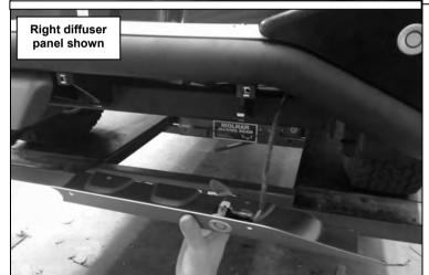
107. Position the diffuser panels on either side of the lift up panel as shown.
