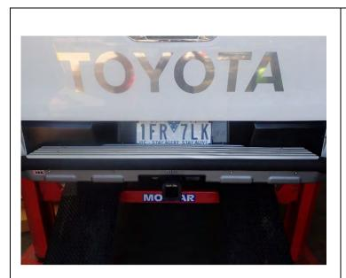
62. Attach the step plate extrusion to the RSTB using 8 M6x1.0x16 button head screws. Proceed to tighten fasteners installed in step 61
