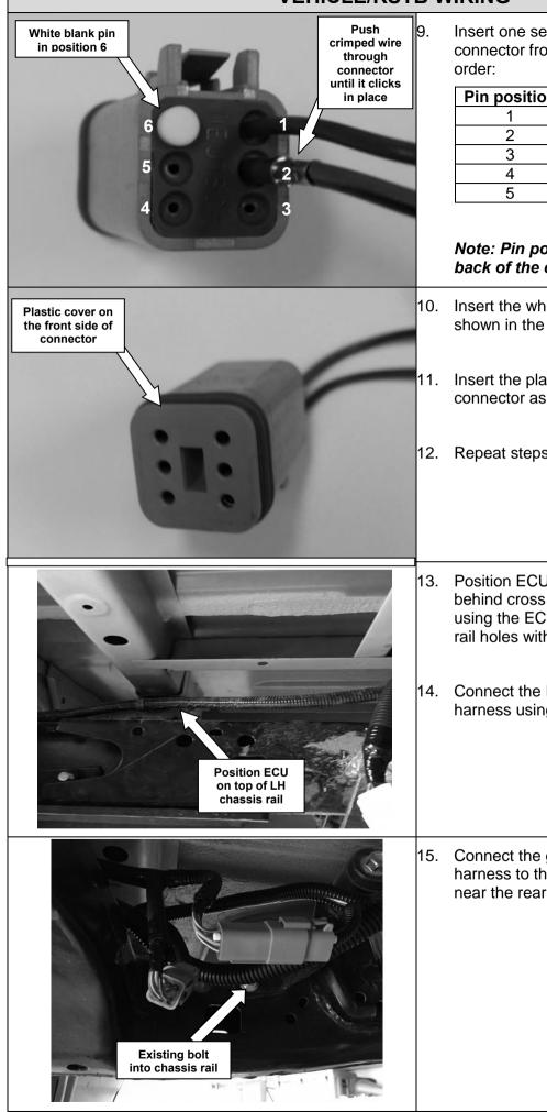
Insert one set of wires into a male 6-pin connector from the back in the following order:
