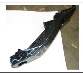
23. Use a white felt tipped pen to mark up the RH plastic bumper retaining bracket: the shaded region is to be cut off.
