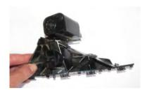
28. Use a hack saw to cut the RH and LH bumper retaining brackets. Once these cuts have been completed the parts should look like the adjacent images.
