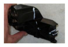
27. Remove the RH & LH bumper retaining brackets from the vehicle. Clearly mark the second cut lines on both sides of the parts as shown.
