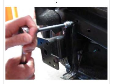
Unbolt the RH & LH bumper retaining brackets.
