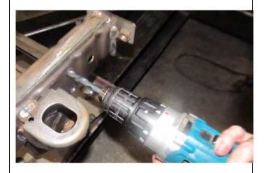
36. Replace the Ø13mm drill bit with a Ø10.5mm drill bit and pass the drill through the Ø13mm holes.
