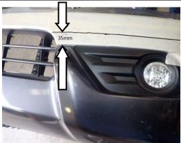
12. Cover the vehicle bumper bar with protective low tack tape in the regions where it is to be trimmed.
