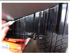
68. Loosely fit the RH and LH wing stone guards to the bull-bar. As shown on the adjacent photo, use a white marker to draw a line on the wheel liner at the lower rear edges of the stone guards.
