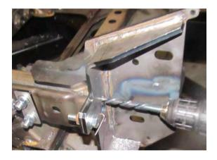
41. Use a punch to mark the two holes in the front of the chassis rail.
