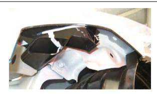
26. Loosely fit the trimmed vehicle bumper. With the bumper in place, use the trimmed edge of the vehicle bumper to mark the second trim line for the RH & LH bumper retaining brackets with a white marker.
