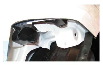
31. Refit the RH & LH bumper retaining brackets and secure them properly with the screws previously removed.
