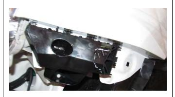
25. Loosely refit the LH and RH bumper retaining brackets. It is not necessary to screw them in place yet.
