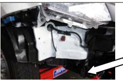
67. Fit the 2 wing stone retaining brackets to the vehicle chassis using the outer bolts holding the vehicle recovery points.
