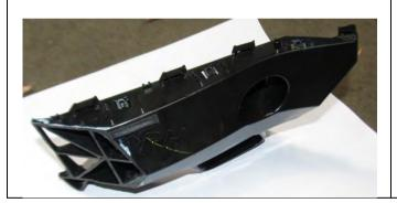
24. Use a hack saw to cut and remove the shaded portion of the bumper retaining bracket as shown in the adjacent image.
