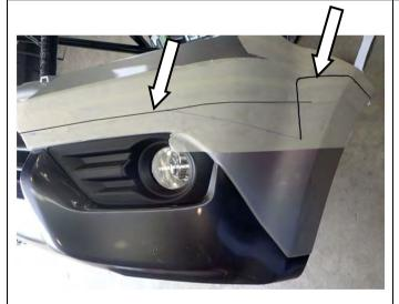
13. Cut the A3 paper template along identified cutting line (Part Number 3789320).
