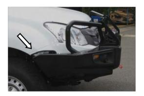
53. Position the bar so that the rear of the wing is parallel with the vehicle fender and lines up with the wheel arch. The nominal distance between the vehicle fender and the bull-bar is 48mm.
