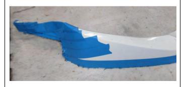
14. With the aid of an assistant, holding the bumper, trim and remove the lower portion of the bumper with an electric jigsaw.
