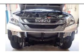
Re-install the cut bumper and grill, refit the scrivits and screw that hold the bumper and grill removed in steps 4 through 8.
