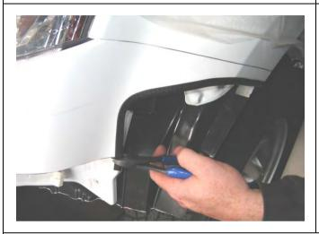
32. Fit the pinch weld, 2 off supplied with the bull-bar fitting kit, to the trimmed bumper as shown. Use side cutters to trim any excess pinch weld.
