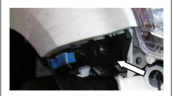
22. Carefully remove the RH and LH plastic bumper retaining brackets. Keep the fastening screws as they will be re-used.
