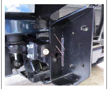
40. Re-use one of the chassis bolts, removed at step 16, to firmly locate the bull-bar mount bracket to the chassis.
