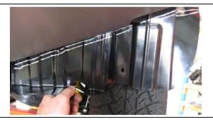
69. Remove the two wing stone guards and mark a second line 5mm above the first line on the RH and LH wheel liners.
