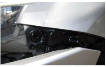
Remove the bumper and mask the vehicle fenders and headlights. Use a spray can to paint the region immediately below the RH & LH vehicle fenders black.
