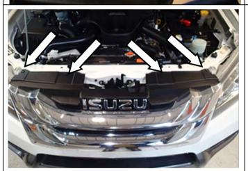
4. Remove and retain the top four scrivets holding the bumper grill.
