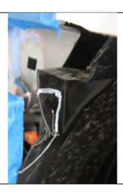
29. Use a white marker to mark the upper wheel liner rectangular cut-outs approximately 60mm high x 20mm deep as shown. Next, use a sharp utility knife to cut out these rectangles from the RH and LH wheel liners.
