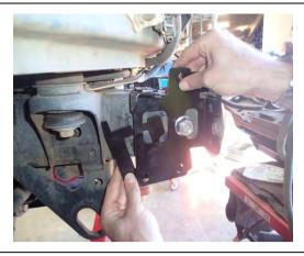
101. Loosely position the outer bracket brace with the packer to the chassis rail. Apply LOCTITE 243 then fit the M16 flange nut to hold it in place. Ensure that the front edge is pushed forward to the chassis flange.
