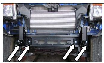
110. Attach the mount bracket to the chassis end plates using 4 x M10 x 30 SEMS bolts into the captive nuts. *Leave loose at this stage.*
