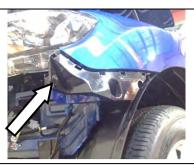
22. Remove screws retaining RH & LH bumper retention blocks to vehicle and remove the retention blocks from both sides and set aside.
