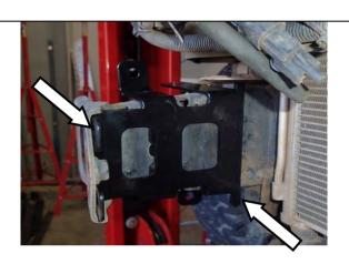
99. Fit the inner brace with the packer to the chassis rail end. Ensure that the front edge is pushed forward to the chassis flange. The brace may need to be tapped to ensure a flush fitment to the chassis is achieved.
