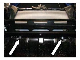
117. Re fit the OE stone shield to the bracket fitted in step 116 using 2 x M10 x 30 SEMS bolts and 2 x M10 flange nuts.
