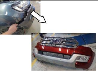
14. Disconnect all sensors and fog lights attached to the bumper and allow them to hang loose.
