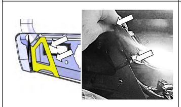
158. On outer LH side of bull bar using 2 x cable ties secure loose loom length and parking sensor connector to brace.
