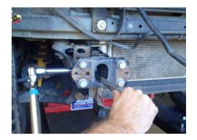
103. Using a spanner to hold the M16 flange bolt, torque the M16 flange nut.
