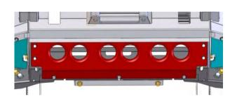
187. Attach the centre stone shield to the mount bracket using 7 x M8 x 25 hex bolts, 7 x M8 spring washers and 7 x M8 flat washers into the cage nuts fitted in step 115.
