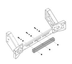
116. Attach the OE stone shield bracket to the chassis mount using 3 x M8 x 25 black bolts, 3 x M8 black flat washers, 3 x M8 black spring washers and 3 x M8 flange nuts.
