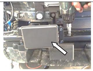
If vehicle is fitted with radar, refer to fitting instructions supplied with adaptive cruise control kit (Part No. 3540190 - purchased separately) for removal and relocation.
