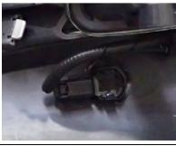
38. If parking sensors are fitted, carefully unclip sensors and sensor loom from bumper bar and set aside for fitment to bull bar.
