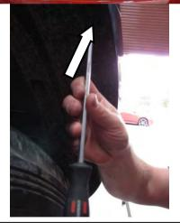
4. Remove all the bumper fasteners along the inside edge of the wheel arches.
