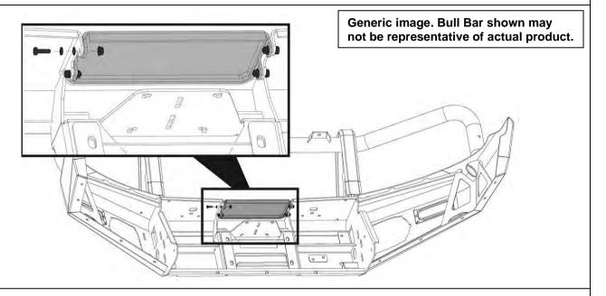
130. Fit the number plate bracket to the top face of the lower-centre pan on the bar using 3 x M6 x 20 hex bolts, spring washers, flat washers and flange nuts.
