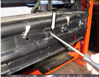
19. Use a screw driver to push the 2 x plastic clips inward from the front cross beam. Do not remove the clips as they will be used later.
