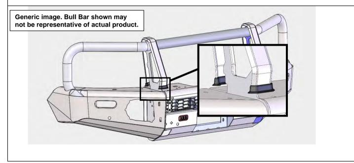
140. From the rear of the bar, slide the rear buffer sections under the rubber mouldings.
