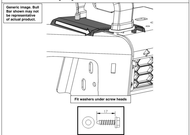
141. By aligning the front buffer with the tongue of the rear buffer, attach the front buffers to the front face of the bar. Ensure each buffer sits flat against the face of bar and is keyed into the top section of the rear buffer.
