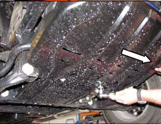
20. Remove the factory under panel and place in a safe place. **Do not completely remove the rear bolts. Leave loose.**
