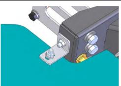
177. On each side of the bar attach the under wing panel to the mount bracket with the wing panel bracket using 2 x M8 x 25 hex bolts, 2 x M8 spring washers, 2 x M8 flat washers and 2 x M8 flange nuts.
