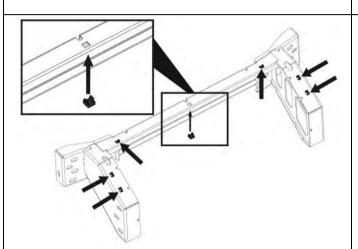
115. Fit 7 x M8 cage nuts into the mount bracket from the inside.
