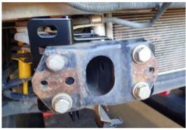
102. Fit 4 x M12 x 35 bolts, 4 x M12 flat washers, 4 x M12 Flange nuts.
