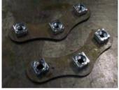
122. Fit 3 x M12 cage nuts to each of the cage nut plates as shown.
