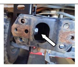
100. Fit the M16 x 35 flange bolt through the front access cut out of the front flange of the chassis.
