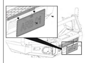
188. Fit the plastic plugs into the square holes in the licence plate bracket. Fit the number plate to the bull bar using the black self-tapping screws.
