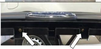
59. Fit the two self tapping screws into the lower section of the grille to join the two parts together as shown
