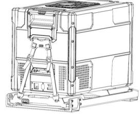
Four holes are provided in the fridge slide to suit the M8 fasteners supplied with the Tie-down kit. On the front tray there are 4 holes, for the taller fridges (69L DZ and 73L) please use the outside holes, and for the shorter fridges (36L, 44L and 60L) please use the inside holes.
