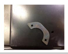
Position locator plate over mounting holes as shown
