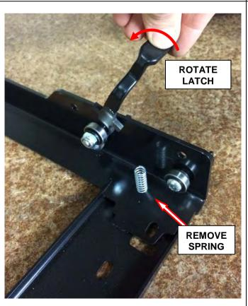
5. Gently release the latch allowing it to rotate into a vertical position as shown.
