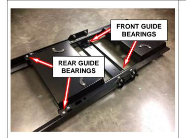
There are 2 pairs of adjustable guide bearings that ensure smooth operation of the fridge slide.
