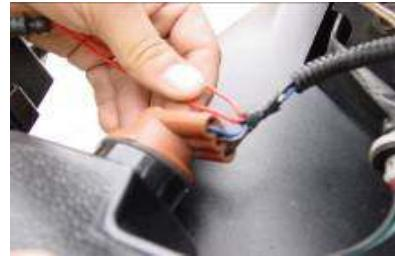
Step 4: take off the turn signals so we can splice the wires to the turn signals and halo resistor.
