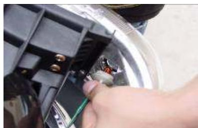
Step 9: Plug and twist the turn signal light into the new headlight
