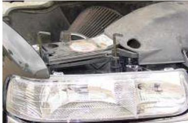
Step 1: remove the two pins holding the headlight housing in place.
